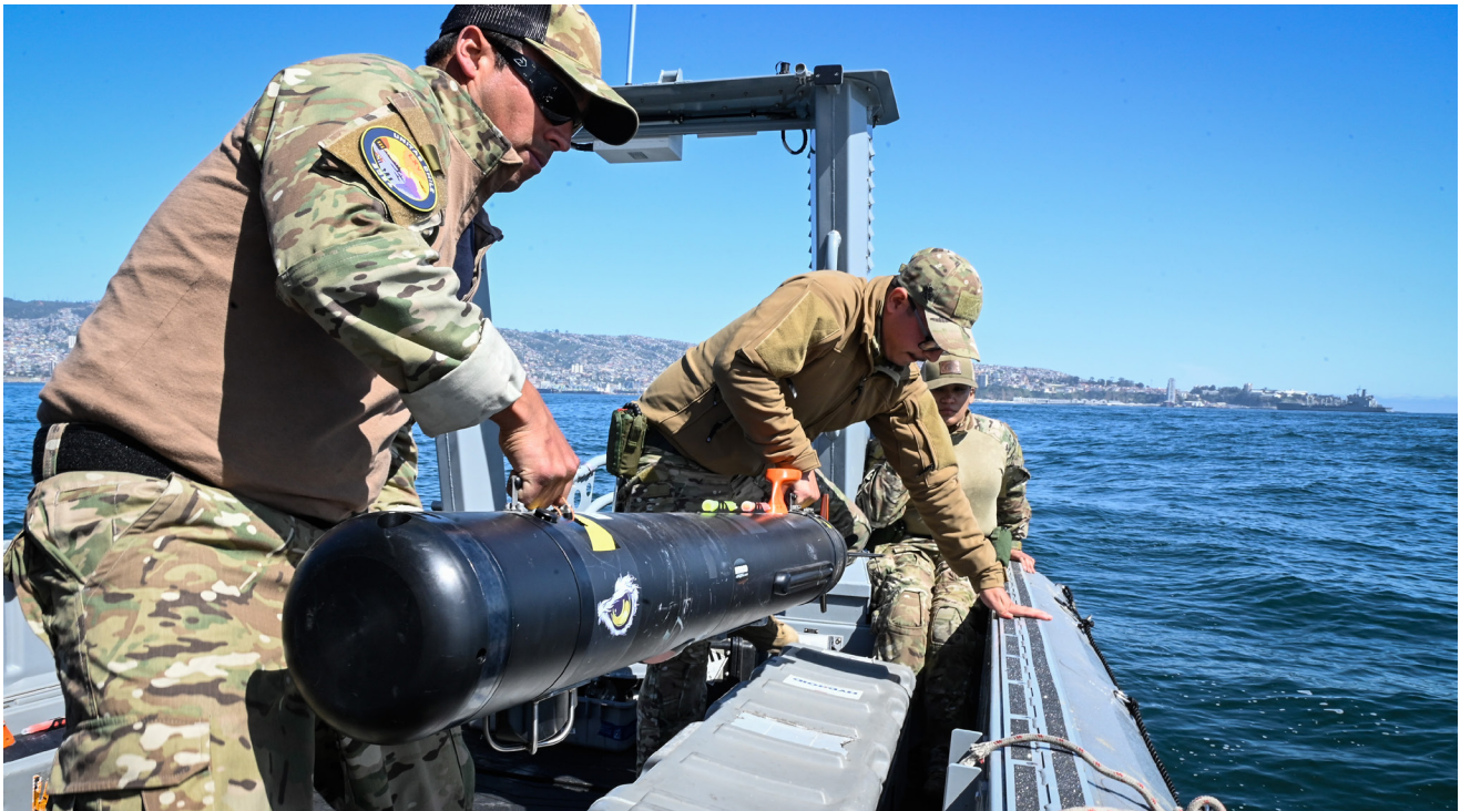
Sailors attached to Explosive Ordnance Disposal Mobile Unit 2 and a Chilean Navy explosive ordnance disposal technician prepare an MK18 Mod 1 Swordfish unmanned underwater vehicle for a marine deployment exercise during UNITAS LXV, September 6, 2024. (Mass Communication Specialist 1st Class Hunter S. Harwell/U.S. Navy via DVIDS)
