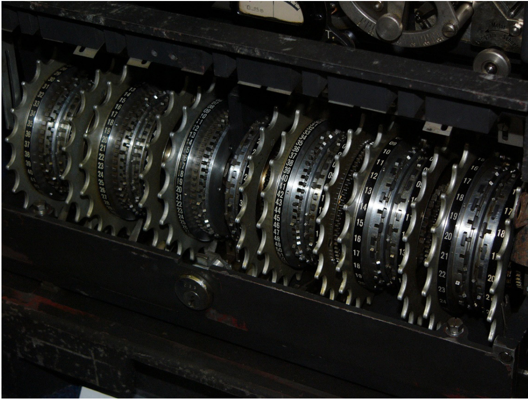
Mechanical rotors of the Lorenz enciphering machine considered effectively unbreakable during World War II. British efforts to break the cipher gave officials access to high-level German communications. Source: Matt Crypto / Wikimedia Commons 36
