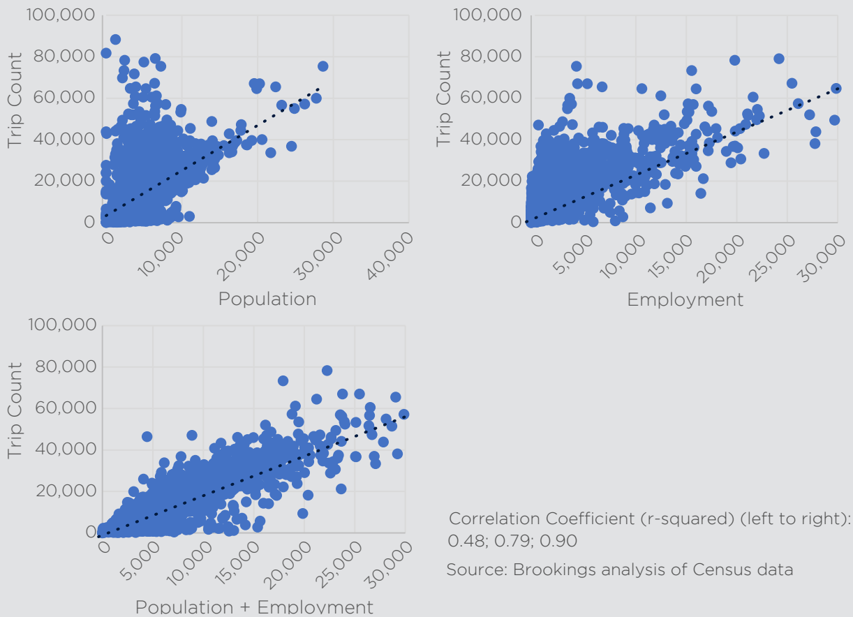
Figure 2. Total trips by tract, cross-tabulated against population, employment, and population plus employment, six metropolitan areas
