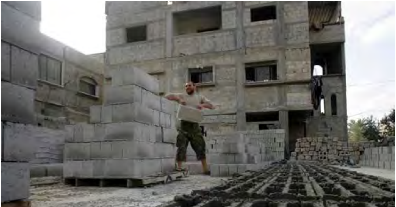
A Palestinian worker stacks bricks made with recycled cement at a brick factory in Khan Younis, Gaza Strip. Due to the Israeli blockade, local tradesmen make recycled cement from crushed rock, concrete, and stone to satisfy a growing demand for building materials. (Warrick Page/Getty Images)
