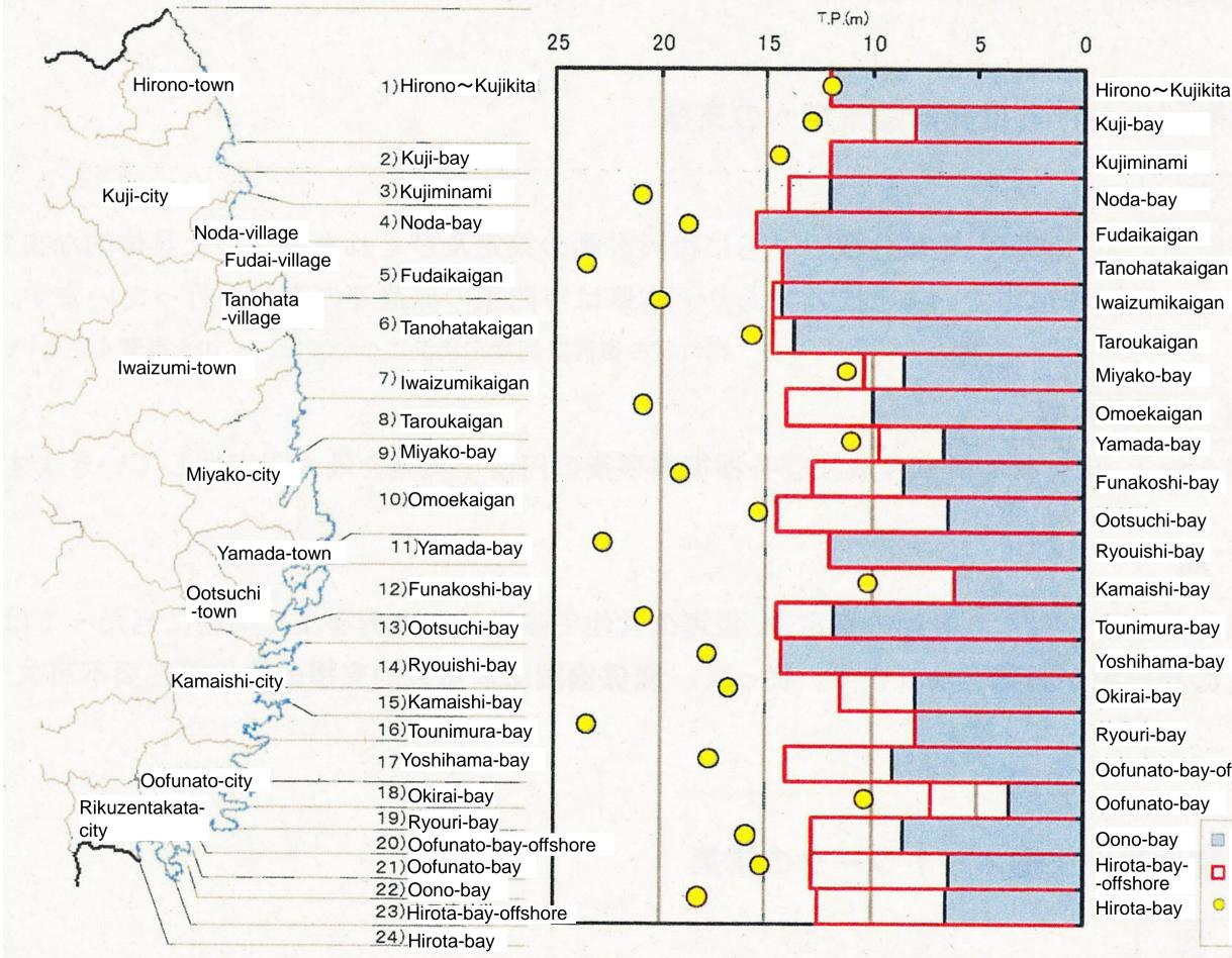
Oofunato-bay-offshore Pre-disaster design level New design level Tsunami trace height
